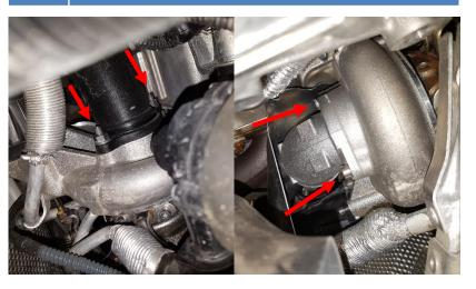
Install the front inlet hose, secure with the included clamp positioned against the bolt heads. Tighten.
