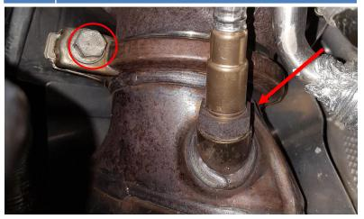
Remove the bracket for the front downpipe secured with 2x 10mm.
