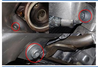
Prom the front turbo, remove the two stud bolts with either 2x M6 nuts, locking each other or with a 3mm Allen key.
