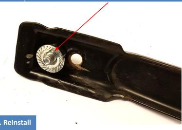
9. Now install the radiator. With the modified brackets. Reinstall all other parts in reverse order.
