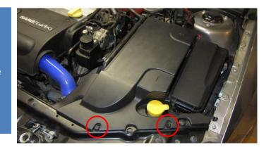
2. Remove the 4pcs 8mm hex head screws in each front inner fender.
