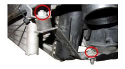
**15.** Remove 2x T25 Torx screws holding the air conditioning filter to the radiator.
