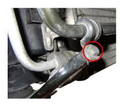
Loosen the 10mm hex nut just a bit, the remove the 10mm hex head screw from the bracket and then turn the bracket out from the car.
