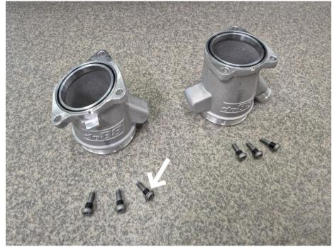
If you have purchased the optional air straighteners, please note that they are leftand right-handed. There are slots machined into the turbo inlet pipes, allowing installation only on the correct side. Refer to the photo for the slot positions.
