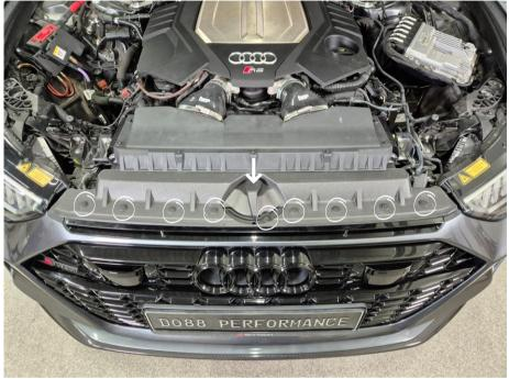
Remove the plastic covers on top of each headlight. Each cover is secured by two plastic tabs pushed into metal clips underneath, and two plastic hooks located at the outer edges near the air filter box.
