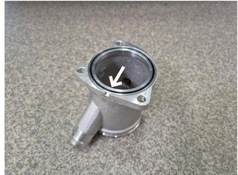
Two different sizes of adapter rings are included—one set for OE turbos and one set for hybrid turbos. Select the correct size for your setup and install the included  $\emptyset$ 62×2 mm O-rings as shown in the photo.
