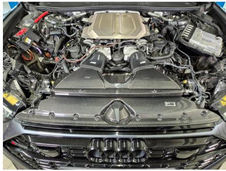
Shape the included large (80–100 mm) hose clamps into an oval form so they fit around the oval connections on the silicone hoses. Position the clamp housings on the underside, with the 7 mm hex screw pointing outward in the same direction as indicated by the arrow in the photo. Slide the clamps about 30 mm onto the hose connections (do not tighten them yet) to allow the carbon fiber air box to be inserted into the silicone hoses without interference from the clamps.
