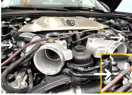
Attach the small metal pipe to the right-side turbo inlet.
