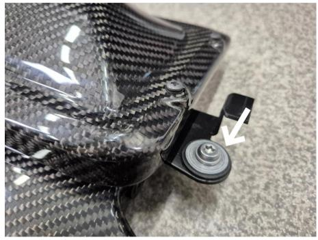
Install the included brackets onto the bottom of the air filter housing. There are two holes on each short end of the housing. Use the provided M5x12 screws and M5 nuts, but do not fully tighten them—leave the screws slightly loose to allow for adjustment.
