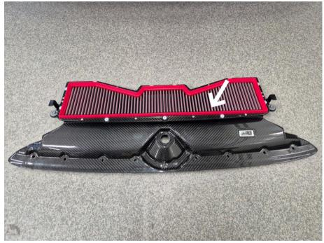
Temporarily install the bottom section of the air filter housing in the car:
