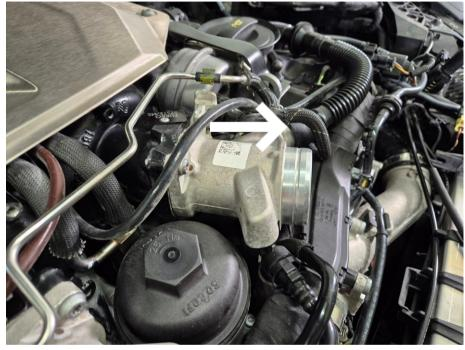
Release the small metal pipe from the turbo inlets by relaesing the metal retaining clips.
