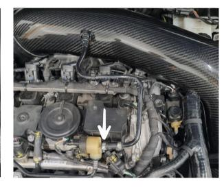
Loosen the spring hose clamp from the coolant pipe and rotate the clamp downwards to make sure it does not interfere with the air filter box.
