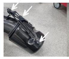
Check the rotation of this metal ring towards the air filter housing by lining up the 3 holes towards the holes in the carbon fiber air filter box. Then install the included rubber sealing strip on the metal ring with the edges on the rubber sealing pointing to the bottom of the air filter box.
