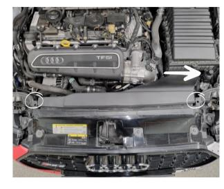
Remove the engine cover, grab the corners of the engine cover and gently lift it upwards.
