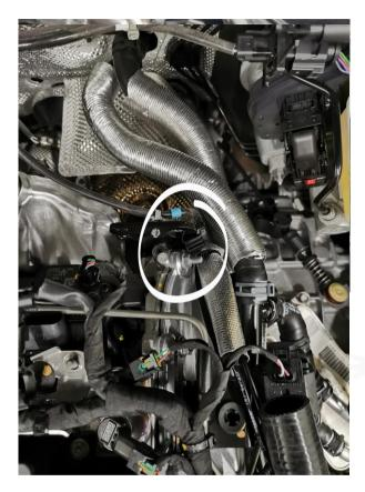
Remove the screw cable holder and fasten it to the bracket behind with included zip-tie.
