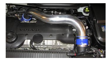
Adjust the pipe and hose positions so the pipe get in a position where you are able to install the included bracket (red on picture but black in pipe kit) fits between cylinder head and inlet pipe.
