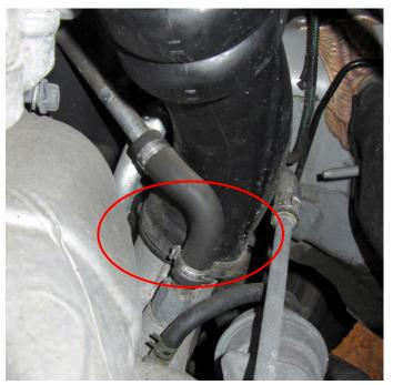
Remove 1 or 2 hoses (depending on car version) attached to lower rear part of the inlet pipe close to the brake fluid reservoir.
