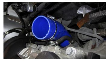
Install the hose amm-pipe on the pipe (with smaller diameter side on pipe) with 2pcs 70-90mm hose clamps installed but not tightened.
