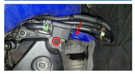
**16.** Install the do88 turbo inlet hose , don't tighten the clamp yet.
