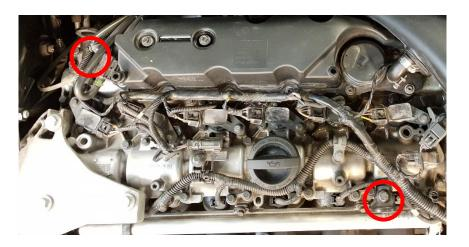
14. Remove 2x Hex 10mm screws according to photo then lift the bracket to the side. Then remove the screw hidden underneath the first bracket and the other screw shown on photo. Now remove this bracket save it if you want to go back to stock at some point. Reinstall all four screws.
