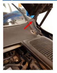
5. Remove six plastic clips and then remove the plastic cover underneath the windshield.
