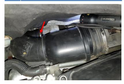
**13.** Remove both engine lifting eyes. 2x Hex 13mm. Save these if you want to go back to stock at some point. Reinstall the screw closest to the firewall now. The other screw will be used when do88 inlet pipe is installed.
