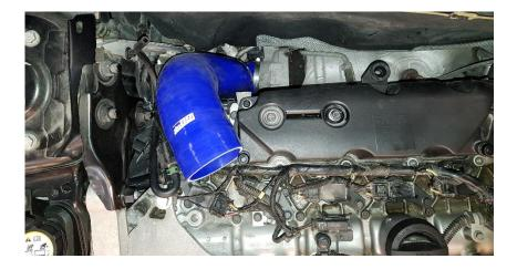
**18.** Install the do88 inlet pipe with the included M6x20 screw and the lifting eye screw removed in step 13.
