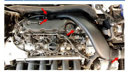
Lift the solenoid out of its bracket. And 11. release the vacuum lines from its bracket on the lower section of the inlet pipe.
