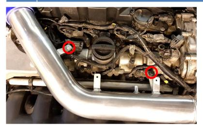
**19.** Check that pipe has clearance between ignition coil connector and also between pipe and the edge of the engine bracket. If you have any interference you will need to gently adjust the bracket(s). Minor deviations may occur since pipe is hand built.
