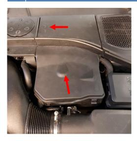
**2.** Remove the windshield wiper arms. Pry away the plastic cover and loosen 2x Hex 15mm nuts.
