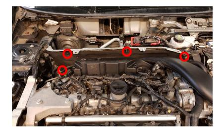
Remove 2x Hex 10mm nuts for the ECU bracket. Then gently lift out the ECU with the cable connection and place it securely on something insolation.
