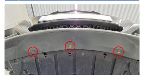
**7.** Remove 4x Torx T30 screws along the top of the bumper.
