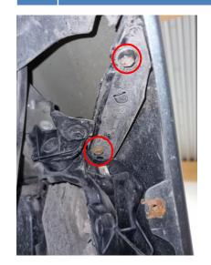
**6.** Remove 3x Hex 8mm screw along the bottom of the front bumper.
