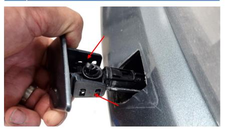
**5.** Remove 2x Hex 8mm Screws in each upper corner of the bumper on both sides.
