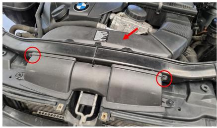
Attach the included intercooler outlet silicone hose on the intercooler. Then install the included aluminum charge pipe from the top (red on this photo).
