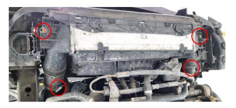
**10.** Remove the intercooler outlet charge pipe. Loosen 1x hose clamp.
