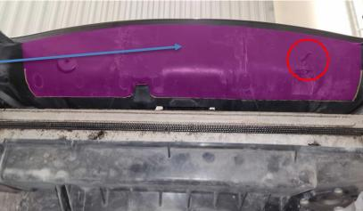
Remove the small plastic trim at the bottom right corner of the radiator. Also remove the sealing along the bottom of the radiator.
