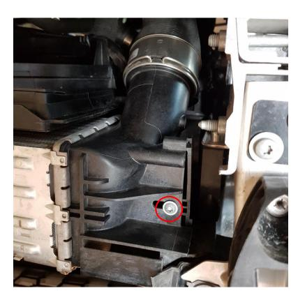
Now install the do88 Performance intercooler with the 2 Included screws. Reinstall all other parts in reverse order.
