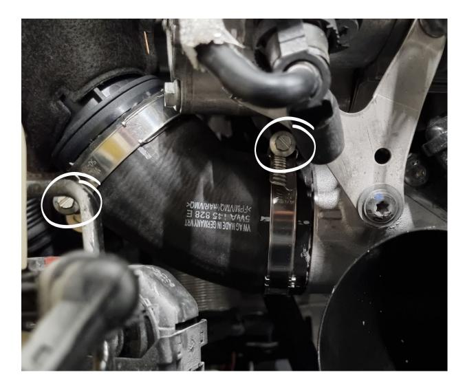
Loosen the coolant hose from the front air filter box duct. Also remove 2x T25 screw to remove the frontal air ducting.
