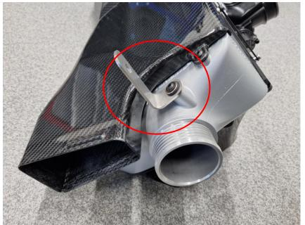
Prepare for both outer intercooler brackets, insert the included M10x70mm screws as on the photo.
