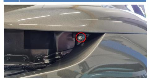
17. Disconnect the left and/or right cable connectors for the rear bumper. Number of connectors depends on equipment installed in the car.
