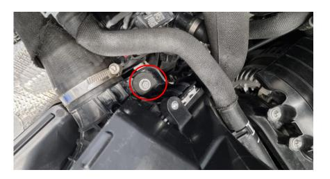
Remove the two clips and washers from the center intercooler bracket. It is a tight space to reach the front clip but can be done using two screw drivers.
