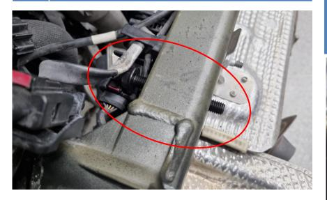
Tighten the throttle body and BOV hose clamps and reconnect the cable connectors disconnected in step 24.
