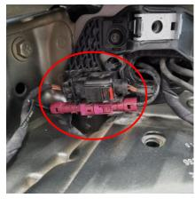
19. Remove the spoiler mechanism. 4x Torx T45 and 1x cable connector.
