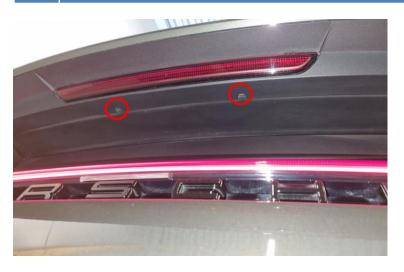
2. Remove the plastic covers underneath the spoiler. Gently pry the three locking tabs with a screw driver.
