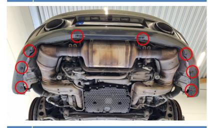
**15.** Remove 2x Torx T30 located top center of the rear bumper cover.
