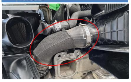
Remove both plastic intercooler side brackets. Push the plastic locking pins rearwards using a 10mm hex socket as on the photo.
