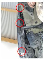
**16.** Remove the final two screws for the rear bumper cover located in the space for the rear lights. 1x Torx T30.
