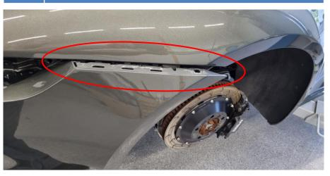
20. On both sides remove the two air ducts.
