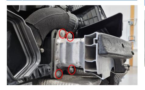
Remove 1x Hex 10mm screws on each side of the intercooler.
