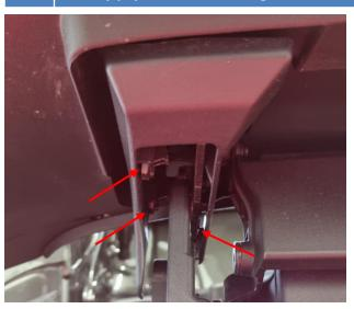
Remove 2x Torx T30 on each side of the spoiler mechanism. Then remove the spoiler by pulling it upwards.
