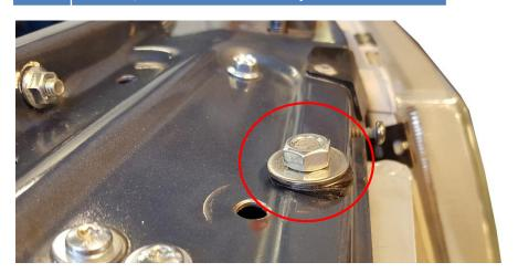
Install the 2 included brackets at the bottom of the intercooler with 2pcs M6x12. Fasten it to the car using the same screws as for the plastic air guide. You can adjust the position of these to get correct clearance between AC/IC/Bumper
