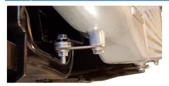
Install the new intercooler pipe and hoses between turbo and intercooler inlet according to photo below.
