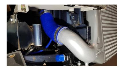
13. Install the new intercooler pipe and hoses between intercooler outlet and throttle body according to photo below.
