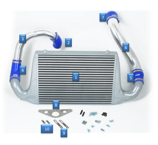
This instruction shows how to replace the OEM intercooler with do88 performance intercooler kit.
