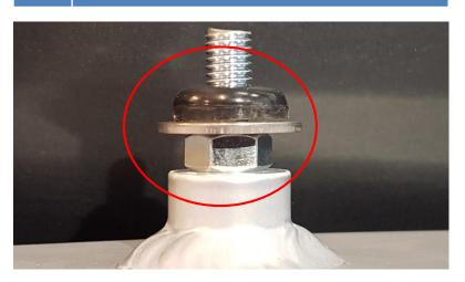
Install the intercooler on the car, gently push the pin screw through the 2 holes you have drilled. Fasten it with the included rubber washer, normal washer and nylon nut.
