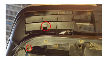
Remove and discard both motors for the head light wipers as those cannot be installed with the do88 performance intercooler.
