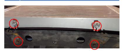
On MY 1987-1993 with Air Condition, fasten the AC condenser to the intercooler with the included brackets, M5 screws, nuts and washers according to picture below. The number of washers needed and their position might vary.
